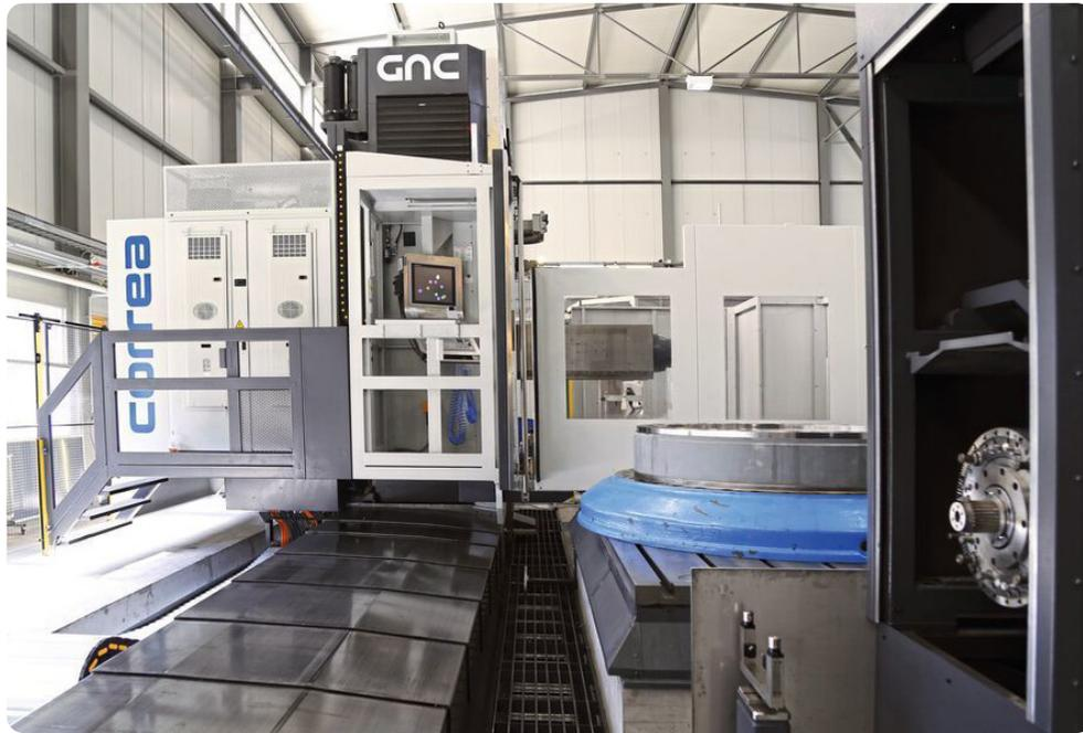
*Hydro's milling machine AXIA is equipped with automatic head changer for two heads.*
